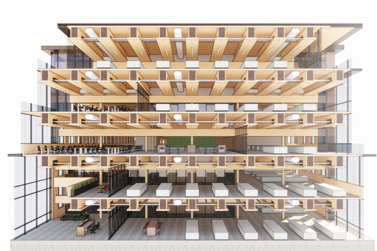
Building cross-section showing incremental adjustment of structural bays and placement of glass walls to create outdoor decks and double-height lobby
