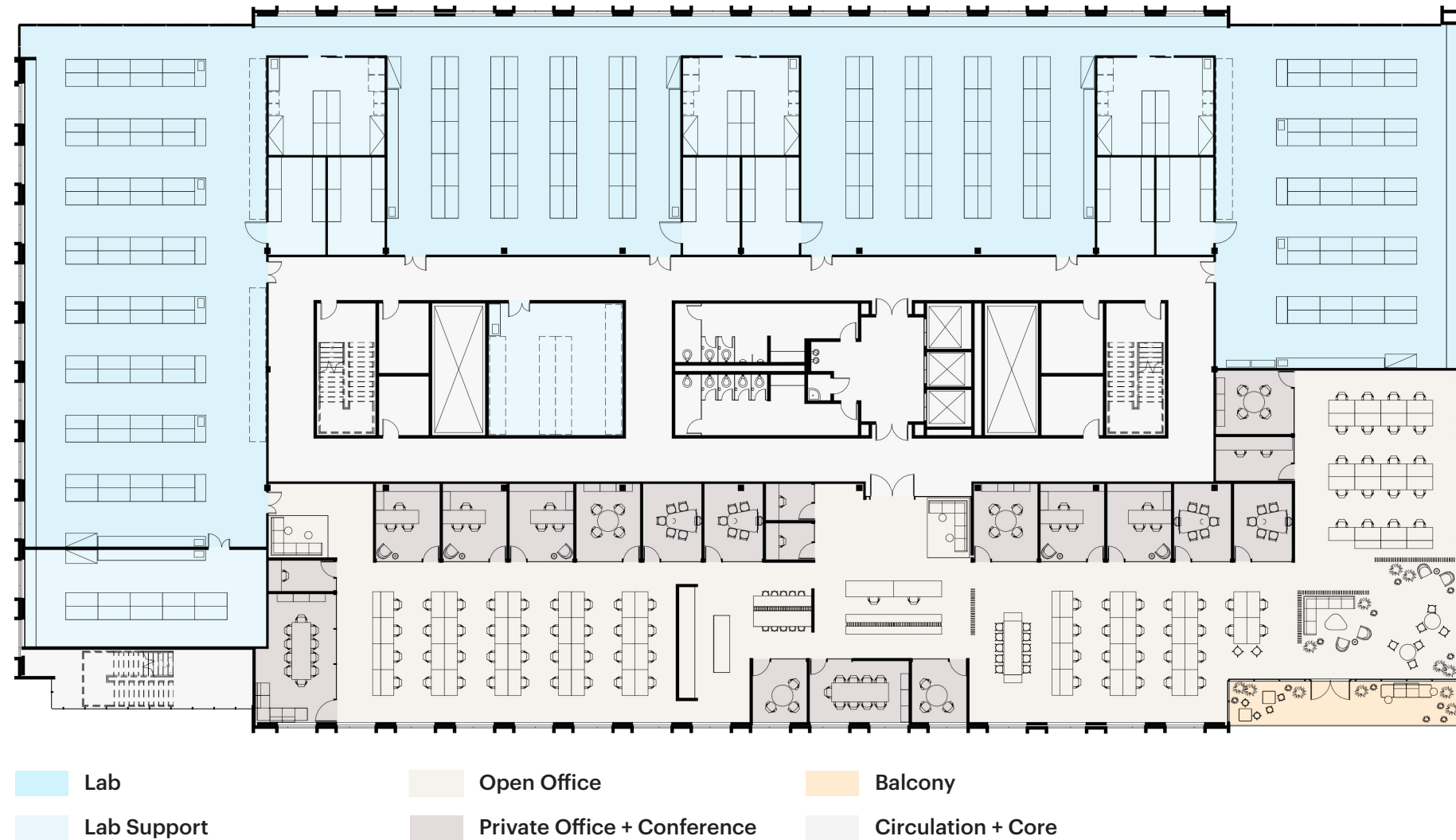
Conceptual test-fit plan of a typical floor, showing 50/50 split between open office and lab spaces
